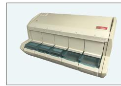
VIDAS<sup>®</sup> is an immunoassay system based upon enzyme-linked fluorescent assay (ELFA) technology for rapid identification of microorganisms.
